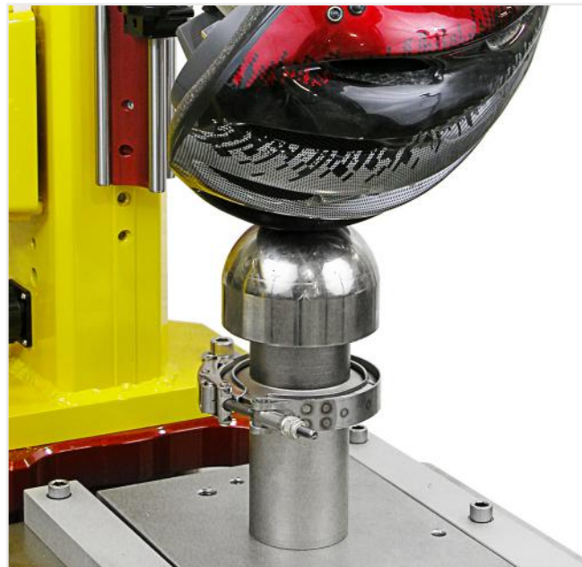
Shown during an helmet impact test
