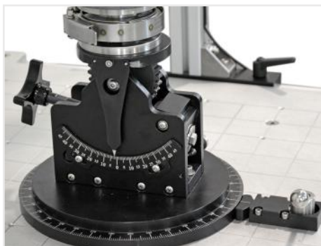
Tilt and rotating headform holder
