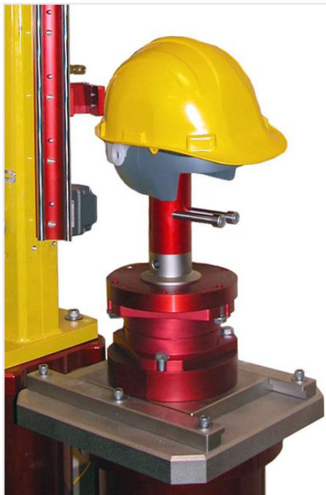
Shown installed on monorail and headform holder for UTM application (P/N: 300_08_HHUTM)
