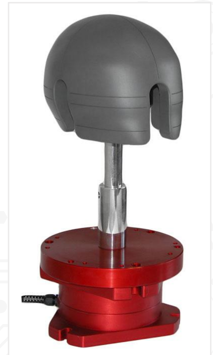
Mountaineer's headform installed on load cell assembly
