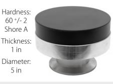
For triaxial testing - P/N: 300\_11\_M60T
