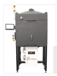
Door shown closed to perform NFPA 1971 conditioning procedure
