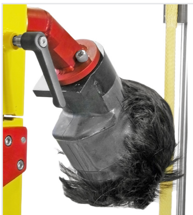
Headform covered with wig included (as per BSI 6658)
